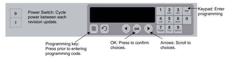
Software updates use the master control display to enter programming codes, scroll to areas to be revised, respond to questions and exit. The control is annotated above. The arrow and OK buttons are illuminated when active.
